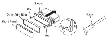
6. Mount the sleeve by inserting it into the opening of the dashboard and bend open the tabs located around the sleeve with a screwdriver. Not all tabs will be able to make contact, so examine the opening to determine which tabs will be most effective. Bend open the appropriate tabs behind the dashboard to secure the sleeve in place.
